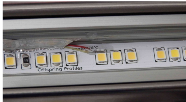
Illustration 3: Thermocouple attached to the LED chip measuring point for this luminaire.
